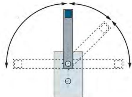
Transducer of rotations in horizontal movement
