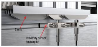
Promixity sensors holders and cams are available as accessories for all sizes of Seventh Axis. The sensors housing kit is in aluminum and features T-Nuts for fixing on the axis profile. The cams are made of steel, with hardened and ground surface. Proximity sensors are not supplied by Rollon.
